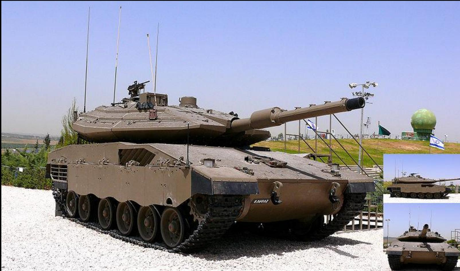
**Weight: 65 tonnes. Seven personnel (four crewmen and three infantrymen) onboard. Armor: classified composite matrix of laminated ceramic-steel-nickel alloy. Speed: 64 km/h (40 mph) on road; 55 km/h (34 mph) off road.**
